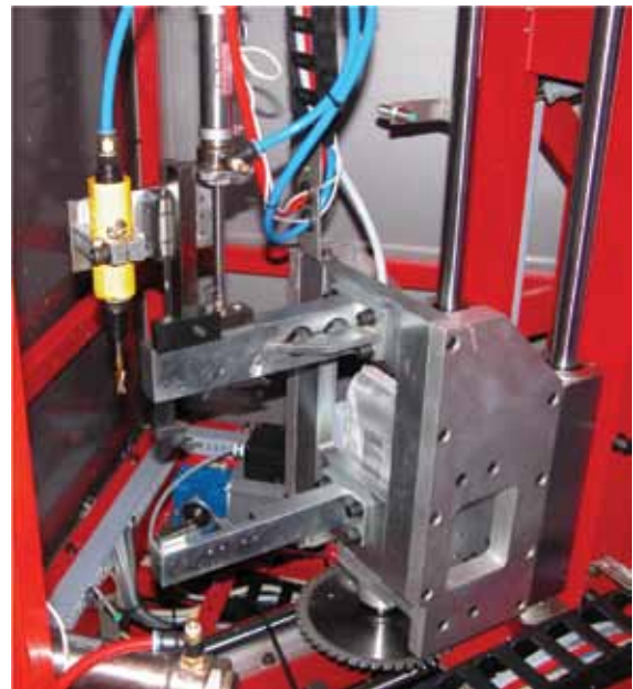
▶ Close-up photo of servo-controlled cleaning tooling, including disc blade scarf knives and vertical drill
