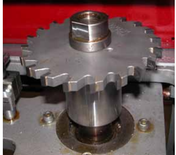
▲ Example of custom cutter installed
