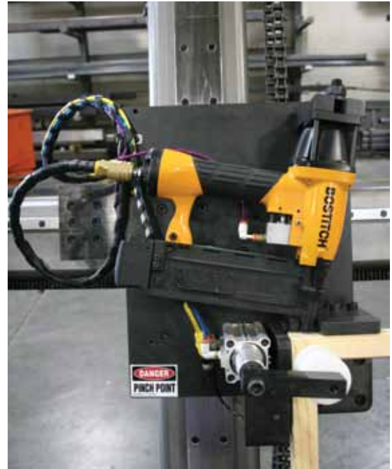
Corner Tool Assembly for sash
