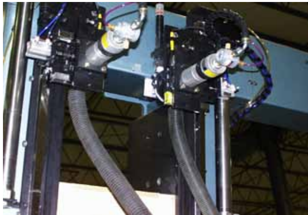
Rear view of the machine showing under mount drawer slide notch routers
